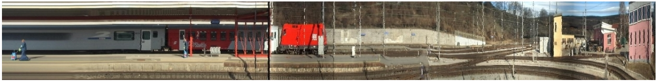
Figure 2: A visual ‘score image’. Acceleration of the train can be observed from left (no movement, i.e. stop at a station) to right: with increasing speed, initially “stretched” objects become more and more compressed.
