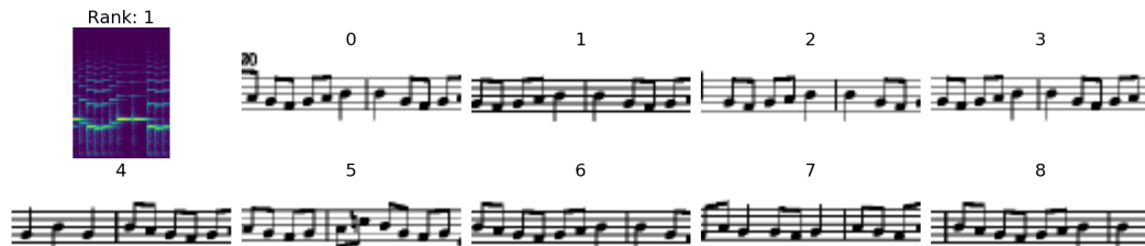
Figure 3: Example of an audio excerpt query and its retrieval results. The number above the spectrogram is the position of the correct result. The numbers above the sheet snippets are the ranks of the respective sheet image snippets in the similarity ordered candidate list.
