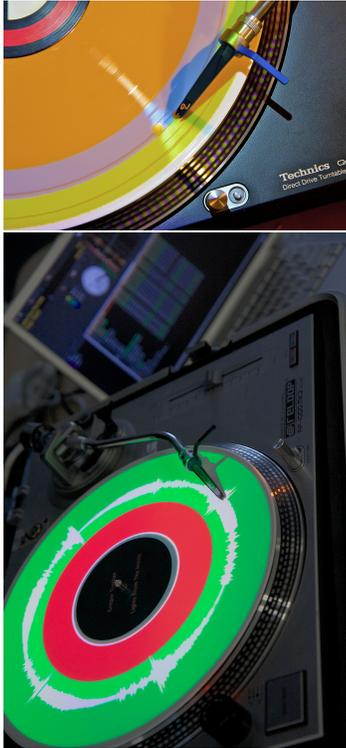
**Figure 1:** DiskPlay visualizes additional information directly on the timecode record of a digital vinyl system, integrating visual output and tangible controller in on device.
